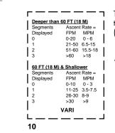
The segments of the Variable Ascent Rate Indicator represent two sets of speeds which change at a reference Depth of 60 FT (18 M). Refer to the chart for segment values.
