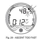
VARI (VARIABLE ASCENT RATE INDICATOR) (Fig. 28c) The Variable Ascent Rate Indicator (VARI) shows how fast you are ascending. When you exceed the maximum recommended ascent rate for the depth you are at (see page 10), the TOO FAST icon will appear flashing and all segments of the VARI will flash (Fig. 29). The flashing will stop and the TOO FAST icon will be removed from the display when your Ascent Rate is slowed below the alarm value.
